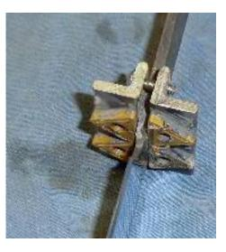
Place the guide on the blade in the desired position and....
