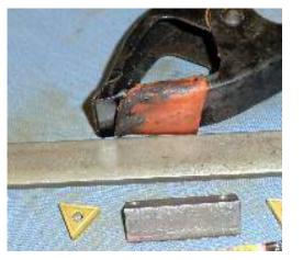
Use a spring clamp to hold some scrap steel and a piece of the angle together such that gravity will hold the inserts in the correct position (side-byside, a long side to the scrap) and dribble a bit of super glue on the edges of the insert to temporarily hold the inserts in place.
