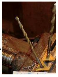
Go to the drill press and first use a #26 drill (which just fits in the hole in the insert) to make a "pit". Then switch to a #32 drill to make a hole precisely centered in the insert's hole.
